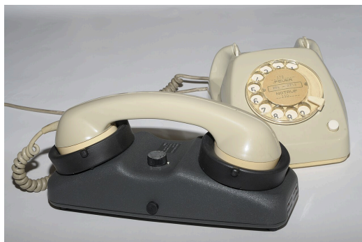
Figure 3: An acoustic coupler [8]
