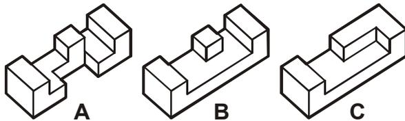
Figure 2. notchable (A), millable (B), non-notchable (C) pieces
