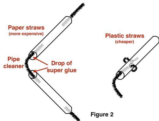
The simple construction method I've found most useful is to use paper straws for the edges, pipe cleaners to join them together at the vertices, and a drop of super glue to hold everything together (Figure 2). The pipe cleaners are flexible, yet hold their shapes, and the short pipe cleaner "tabs" at the ends allow the easy construction of three dimensional models.
